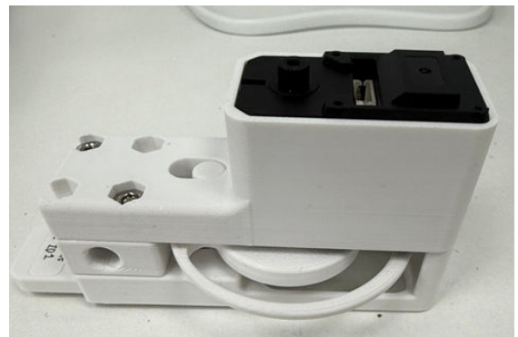
The team's pinch valve, assembled. The servo body is on top, with the valve's lower parts under its arm.
