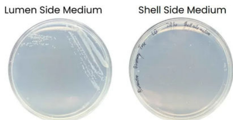
Figure 3. Containment check. Lumen-side medium (left) and shell-side medium (right) on LB agar after 24 h at 37 °C. The lumen plate grew colonies; the shell plate grew none.
