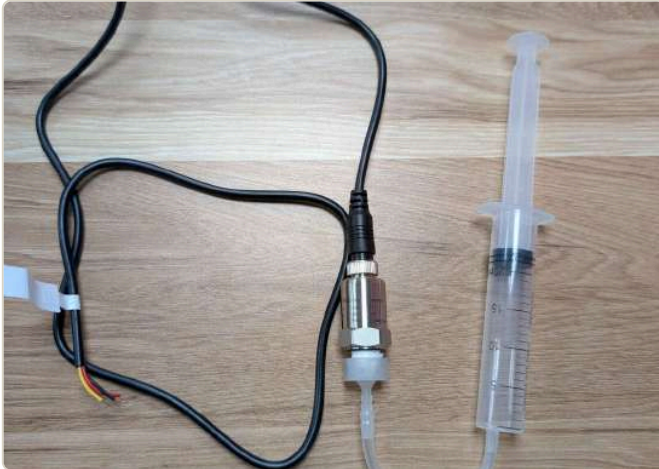
10 July: transducer and Luer line before fitting
