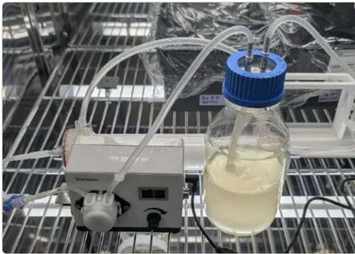
Prototype I loop on the bench: pump, membrane cartridge, reservoir
