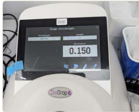
The benchtop BioDrop reading 0.150
