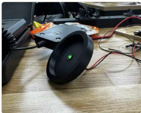
The printed jig: one LED lit at the centre, lux meter behind
