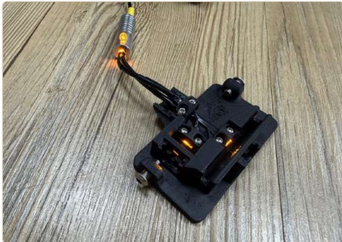
12 October: the newer photometer, light almost against the cuvette
