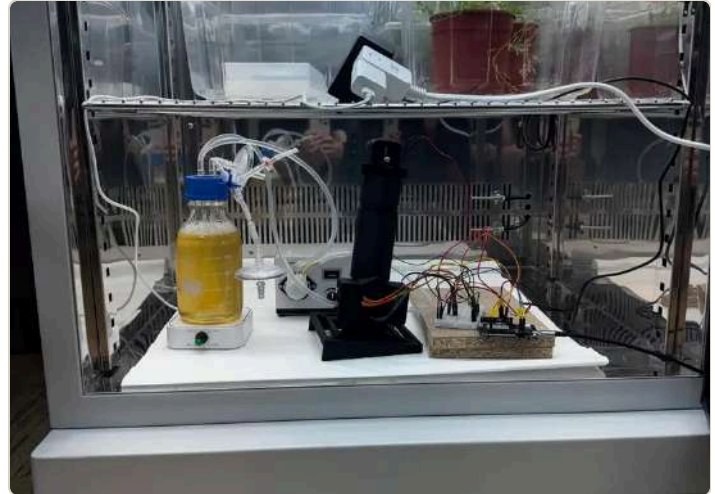
The photometer column on its wedge inside the chamber
