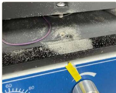
The housing on the shaker: debris around a torn hole in the bottom plate
