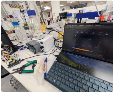
19 July: photometer in line on the loop, live data on the laptop
