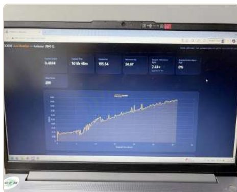
Dashboard at 1 d 6 h 46 m, 291 points: OD600 0.4834, ratio 7.33x
